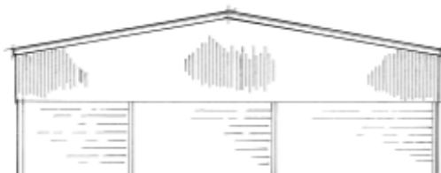
END NORTH Yorkshire boarding over blockwork walls
