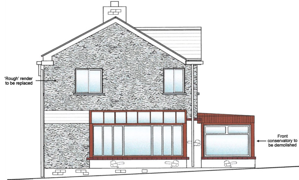
Proposed re-rendering of external elevations, removal of front conservatory and erection of new front porch. Removal of aluminium windows to be replaced with new Heritage 'wood grain' uPVC casement windows. Erection of 1.4m random stone boundary wall. 'Pennyard House' East Street, Barwell North Somerset BS29 6BW
