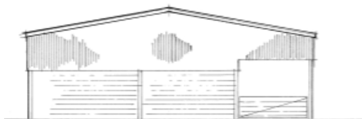
END SOUTH Yorkshire boarding over blockwork walls
